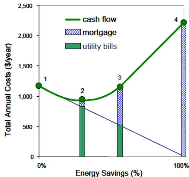
**Figure 2.4 – Cost to reduce energy consumption from a base case (Christensen 2004).** From a base case (point 1) there are initially cost-effective methods to reduce energy consumption, but those energy saving methods eventually become more costly (points 2, 3, and 4).
