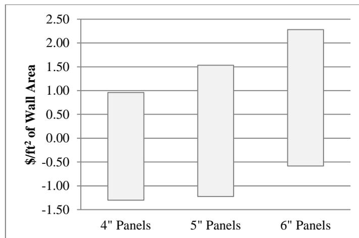
**Figure 3.16 – Relative 60-year present value in dollars per square foot of wall area due to increasing panel thickness from 2.5 in (63.5 mm) on each side for Chicago, where the range of values for each bar represents a discount rate of 0-5%**
