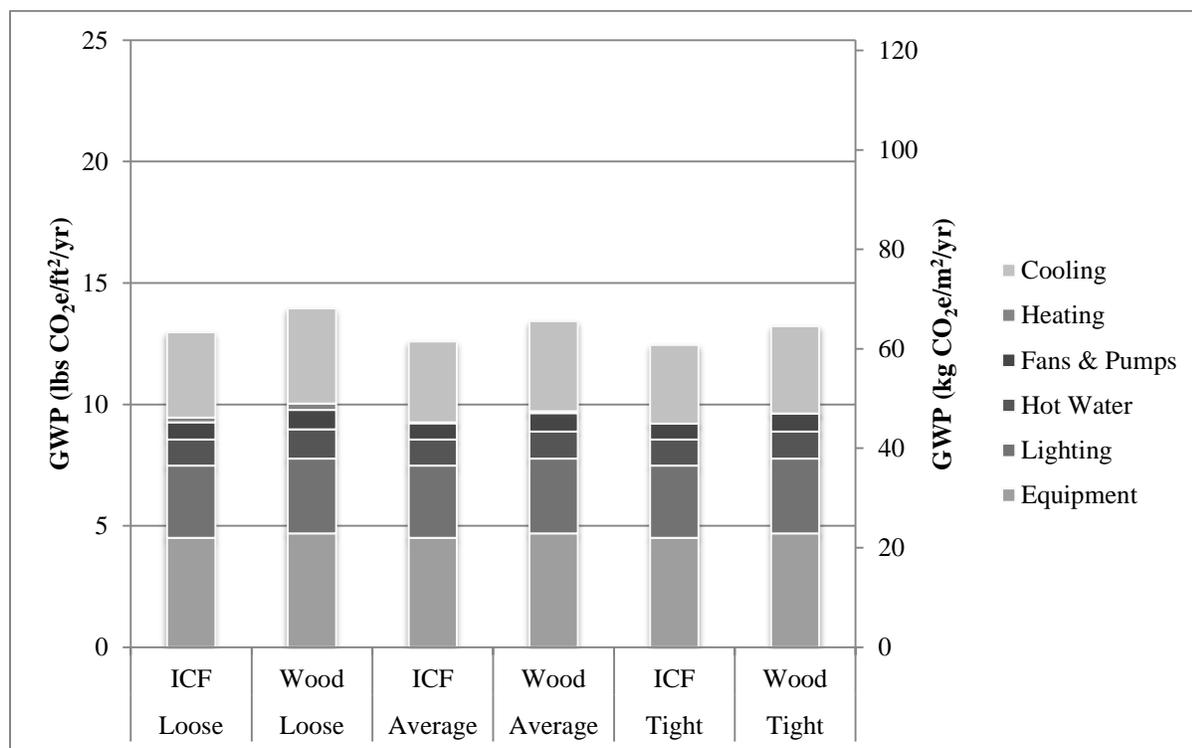
Figure 3.25 – GWP associated with annual energy use and normalized by gross floor area for the multi-family buildings in Phoenix, separated by air tightness and energy end-use
