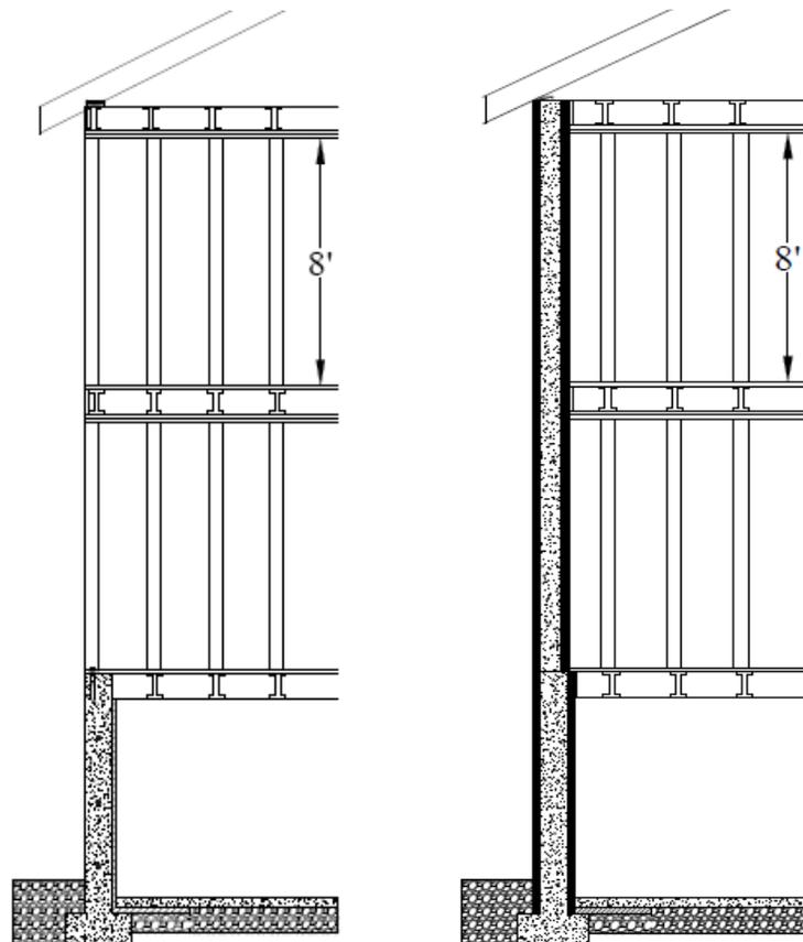
Figure 3.3 – Structural design of the light-frame wood and ICF single-family houses for Chicago
