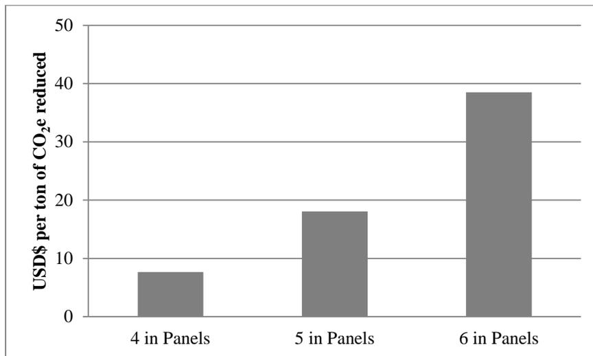
**Figure 3.17 – Life cycle cost per ton of CO<sub>2</sub>e reduction by increasing panel thickness for Chicago**
