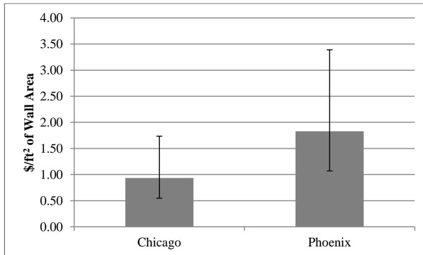
**Figure 3.12 – Present value of energy savings over the 60-year lifetime of the ICF wall compared to wood construction for 2,400 ft<sup>2</sup> (223 m<sup>2</sup>) single family house**
