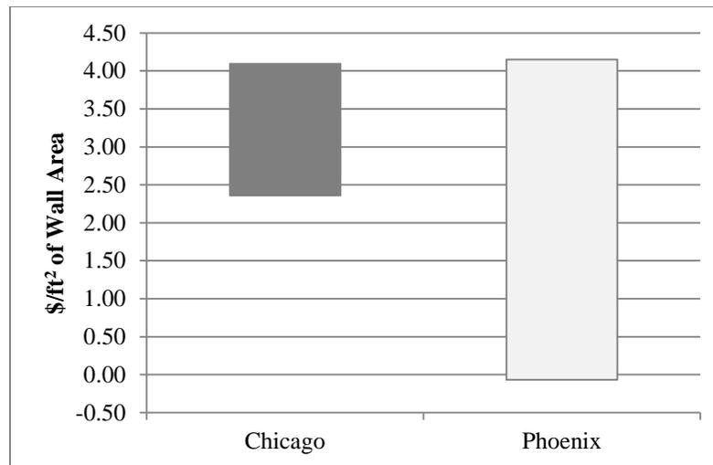
**Figure 3.13 – Total life cycle cost of ICF relative to light-frame wood construction for single family house**
