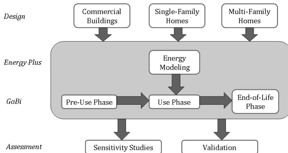
Figure 2.2 – Methodology of current project with associated software
