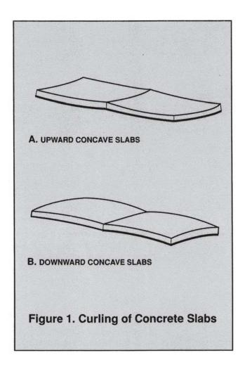
related to poor curing and rapid surface drying; and anything that increases drying shrinkage will tend to increase curling.
