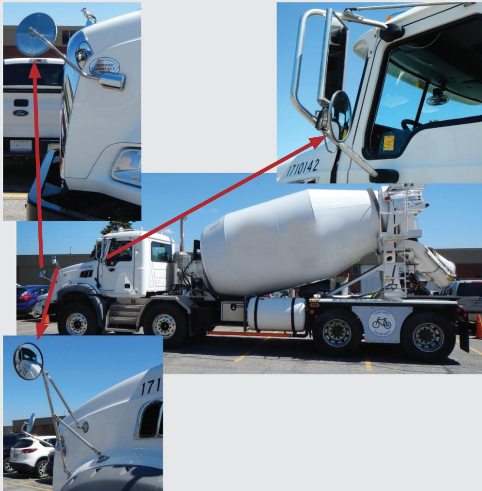
The goal of this mirror configuration is to adjust the mirrors so that objects can transition from one mirror field-of-view to the next, thus allowing the Ready Mix driver to track the movement of vehicles and pedestrians around their truck.
