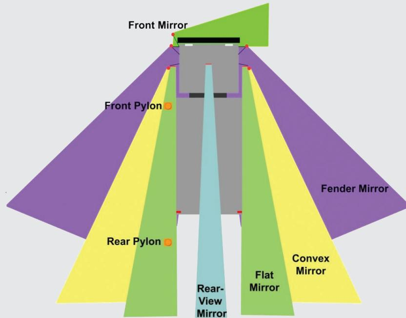
(Note: The rear view mirror shown here would not necessarily apply to Ready Mix trucks, however might apply to other vehicles in a Commercial Fleet.)
